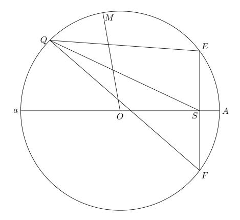
Draw now ESF perpendicular to AO, then the arc AE, which has the excentricity OS for its cosine, may be called the arc of excentricity; we shall denote it by e; while AQ, the arc defining the planet's position,<sup>77</sup> may be denoted by p. Having joined EQ, FQ, it is seen, by mere inspection, that the mean anomaly<sup>78</sup> AEQS is half the sum of the two circular segments cut off by the chords FQ, EQ, or that
