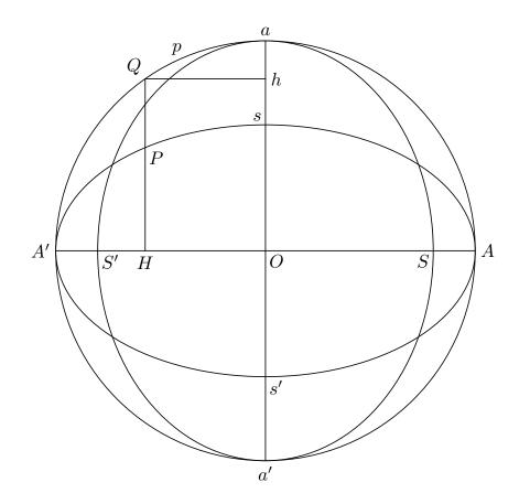
From those we easily get the tangent of the true anomaly ASP, and thence the distance SP. Here the great part of the labour is in finding the logarithm of SH, the angle HSP from its log tangent, the log secant from the angle, and SP from its logarithm; that is to say, in using the tables of the logarithms of numbers, and of circular functions to a considerable number of decimal places. This labour, repeated for each of the twenty thousand cases to be tabulated, rises to a formidable total.
