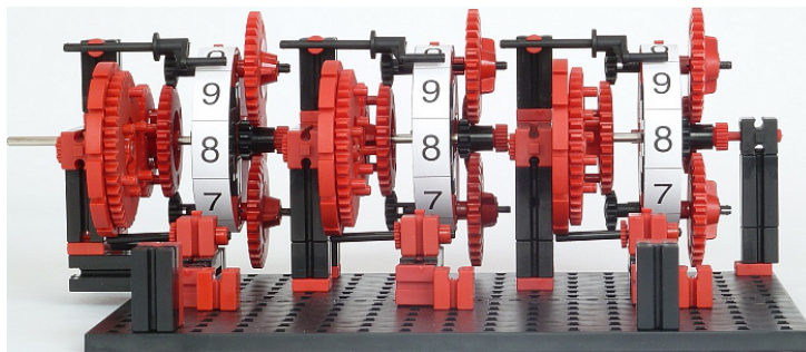
Figure 23: Püttmann's simplified reconstruction of Chebyshev's adding machine. ( https://fischertechnikblog.wordpress.com )
